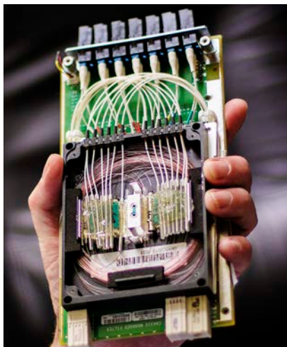
Ciena's CN 2150 passive optical multiplexer, a later generation of the MultiWave 1600, which in 1996 increased Sprint's network capacity by 1,600 percent. © Spencer Trask/Julie Allocco
